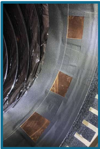
Figure 5a: Coupons in air stream before (left) & after (right) 3,400 hours of run time
